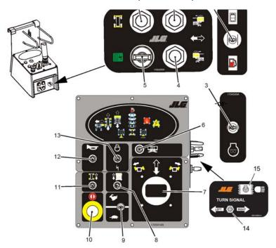
**Figure 3-3. Platform Control Station**
