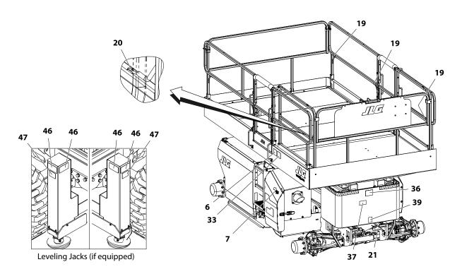
Figure 5-10. Decal Installation - Sheet 2 of 2 (CE/AUS)
