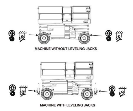
Figure 3-6. Lifting and Tie Down Chart (Sheet 2 of 2)
