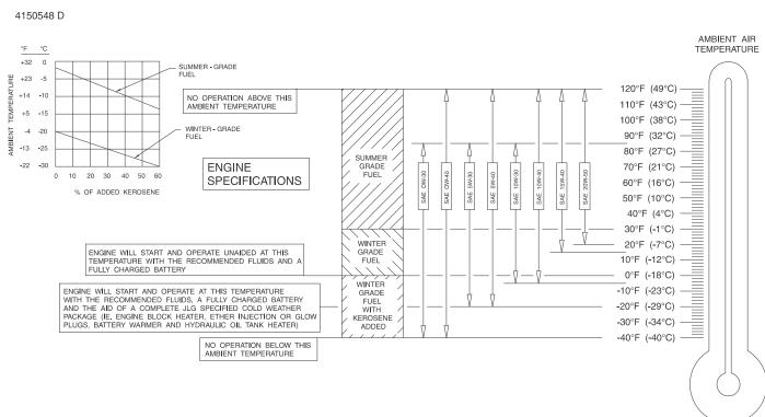
Figure 5-1. Engine Oil/Diesel Fuel - Operating Temperature Specifications - Deutz - Sheet 1 of 2
